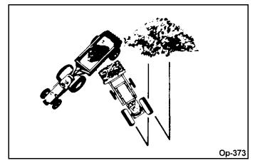
Do not roll bucket over and attempt to backgrade. This type of use can cause severe overloading of bucket cylinders when fully extended, possibly causing bucket cylinder rods to become bent.
